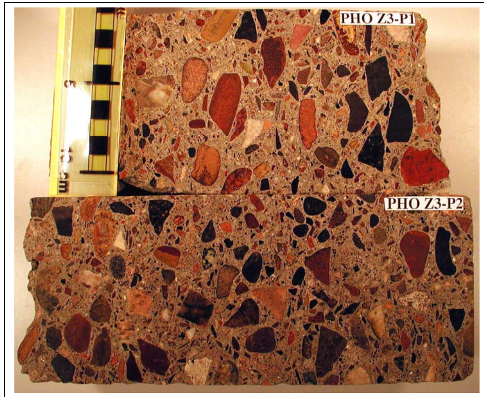
Fig.1 continued: Photograph of polished surfaces showing the size, shape, color and distribution of the coarse aggregate in the concrete.
