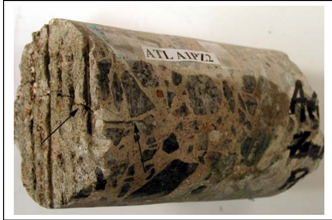
Fig.5: Core A1-Z2 showing a crack crossing the grooved surface, indicated by arrows and extending about 2 inches (50 mm) into the concrete.
